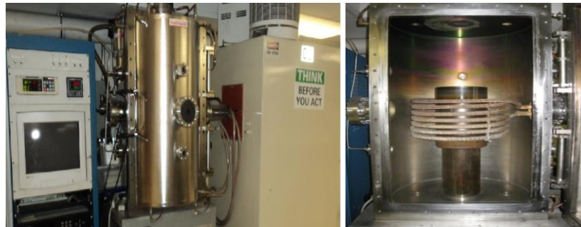
Figure 3.1 Hot Wall RF reactor outside (left) and inside (right) of growth reactor showing induction coils and graphite crucible.
